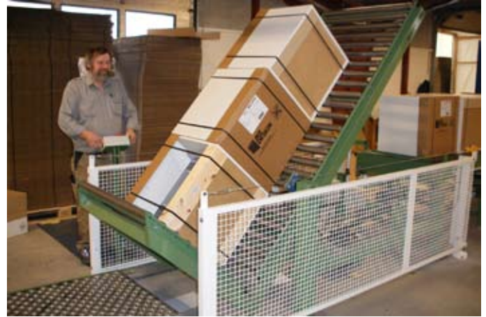
The stack is formed using the tilting unit and then pushed onto the transfer cart.
