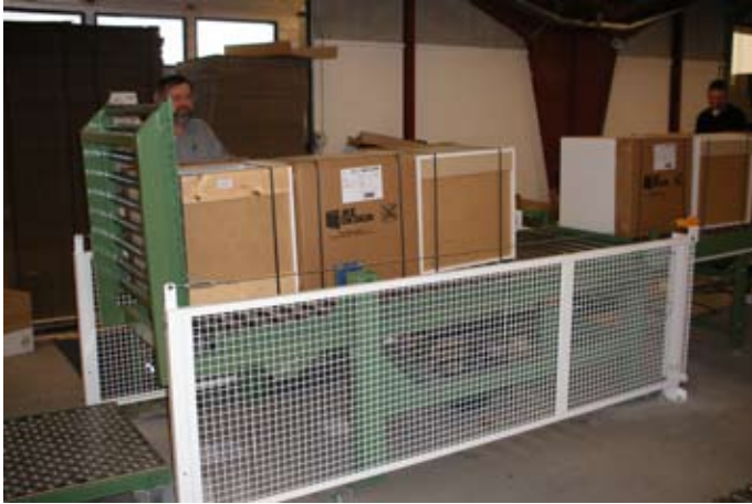
The operator will arrange the cabinets before tilting them 90°
