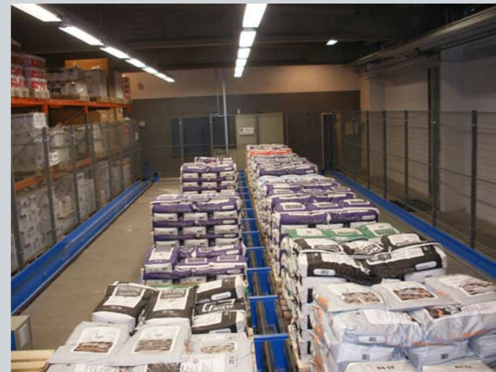
The approach conveyors can all hold two pallets with one type of product.
