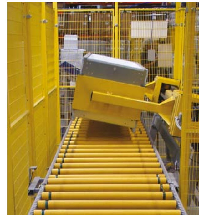
The cabinet is turned by means of a pressing unit which adjusts automatically to the height of the cabinet.
