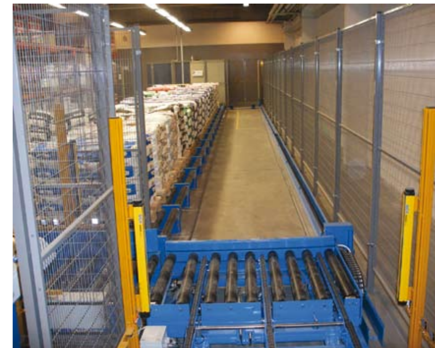
The transfer cart stands ready to receive another pallet to be fed into the order picking system.
