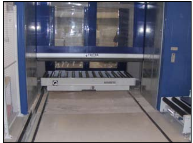
The transfer cart is on its way through the lock to pick up another stack of plates for spray painting.
