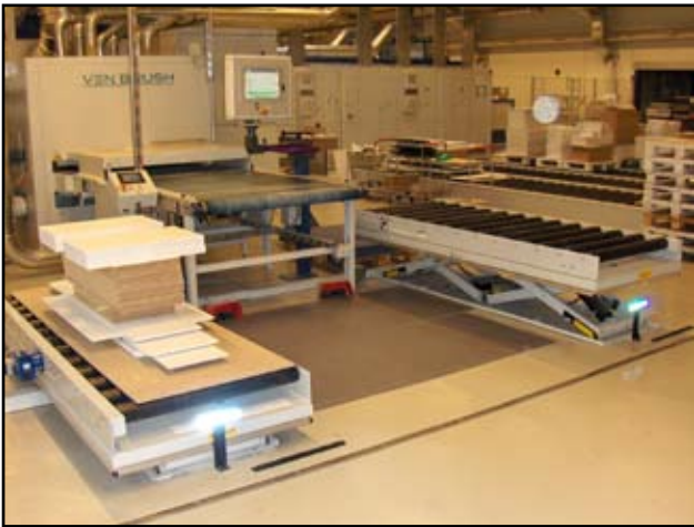
The two lifting tables at the in-feed end of the spray plant serve a dual purpose: to ensure the operator works at the correct ergonomical height, and that there will always be items ready for feeding the spray plant.
