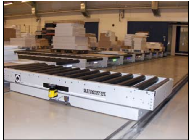
The transfer cart which brings stacks for painting to the operator at the spray plant runs in an unfenced area as the scanner on the cart will bring the cart to halt if it detects an obstacle.
